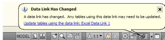
If changes are made to the data in the external file, AutoCAD displays a balloon notifying you of the changes. You can then quickly update the table by clicking on the link inside the balloon.
