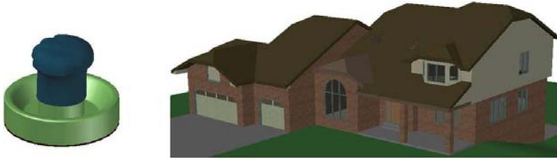
The air hockey paddle has several cylinders, an array of boxes, a sphere at the top and even an inverted cone of removed material. The house has many boxes and wedges, and a cylinder.
