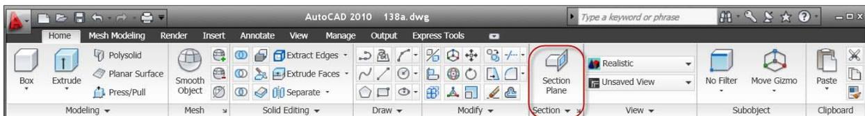
You can define a section plane using various methods. You might want to pick points or select from standard orthographic options. If you choose the Orthographic option, you can then specify front, back, top, bottom left or right. AutoCAD automatically creates a section plane aligned with that view. You can then select the section plane and use grips to flip its direction, or change its location.
