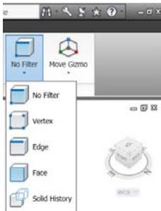
If you leave the subobject selection filter as the default, No Filter, your selection is less predictable. For example, if you pick on the corner of a face, AutoCAD could potentially select the face, edge, or vertex. When you use a window selection, it selects all the subobjects that fall within the window, which may or may not be what you intended. Set the subobject selection to Face to select the faces for making the narrow finger impressions.
