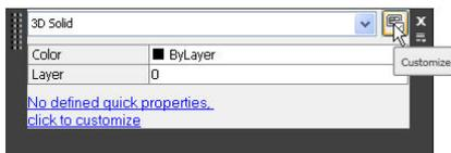
The Customize User Interface (CUI) dialog box is displayed and the select object, a cylinder in my case, is automatically added to the Quick Properties object type list (if it wasn't already there). Now you can simply turn on the properties you want QP to display for that particular type of object.
