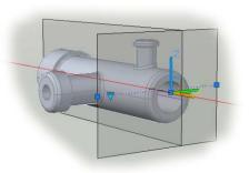
Once the new section plane has been created, you can use the tools in the Generate Section/Elevation dialog to create a new two-dimensional block that shows the 3D model projected onto the section plane and place that block into your drawing. Again, if you subsequently make changes to the 3D model, you can use the tools in the Generate Section/Elevation dialog to replace the block with an updated version.
