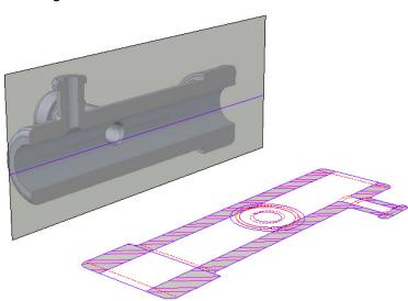
If you subsequently make changes to the 3D model, you can repeat this process, but instead of inserting a new block, you can choose Replace Existing Block and then select the block you previously created. AutoCAD immediately updates the block to reflect the changes you made to the 3D model.
