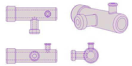
As is true with views created using section planes, if you subsequently make changes to the 3D model, you can replace the existing blocks to reflect the changes you made to the 3D model.
