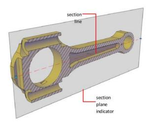
If you subsequently make changes to the 3D model, you can easily update the blocks created based on those section planes to quickly update the two-dimensional views to reflect those changes.
