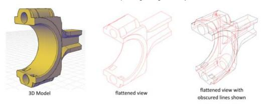
Once the model is set up the way you want it to be captured, select the Flatshot tool from the extended Section panel on either the Home or Mesh Modeling ribbons. AutoCAD displays the Flatshot dialog. This dialog lets you control various aspects of the creation of the 2D representation.
