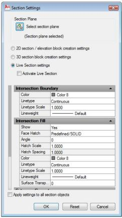
By default, the settings only apply to the current section object. If you select the Apply Settings to All Section Objects check box, however, the settings will apply to all section objects in the drawing.
