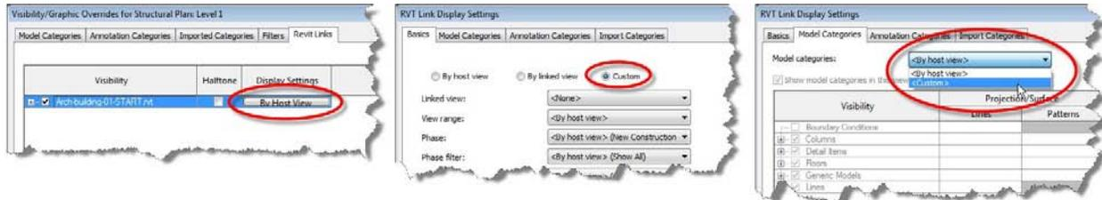
If you click the By Host View button, however, Revit displays the RVT Link Display Settings dialog. This lets you control the visibility graphics for the linked file. To control its settings separately from the current project file, you need to make two changes. First, on the Basics tab, change the setting from By Host View to Custom.
