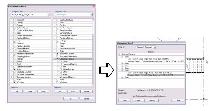
Interference checking can be performed between structural, MEP, and architectural objects. In this example, the resulting report shows that a structural column is interfering with a staircase.
