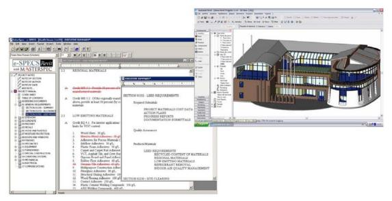
The ODBC standard is used to integrate the Revit building information modeler with data-centric applications such as e-SPECS for specification management.
