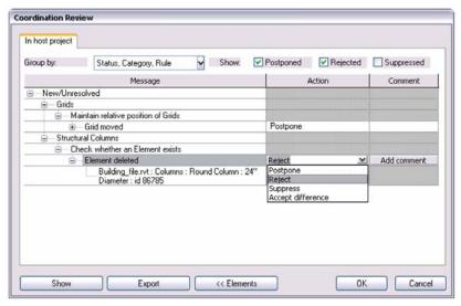
Modifications made by the engineer or the architect on monitored elements can be reviewed in a convenient and accurate format.
