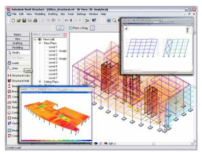
Revit Structure links its analytical model to several structural analysis and design software applications.
