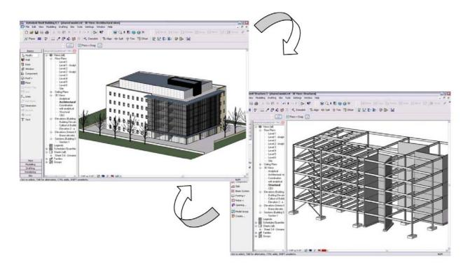
Cross-linking architectural and structural models is the common method of sharing design models in Revit.
